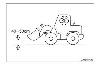
When the bucket is loaded, avoid sudden swinging or starting. Overloading is dangerous. Make sure the load does not exceed the permissible level.
